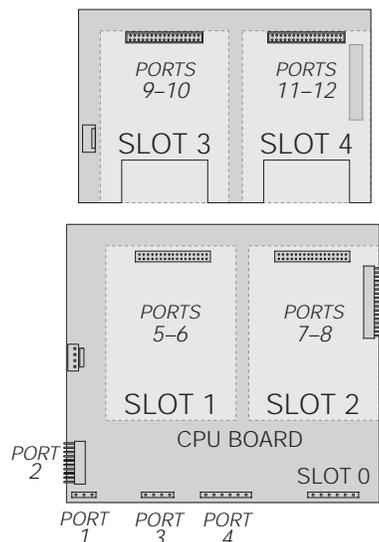
Figure 2-10. Serial Port Assignments, Two-Card Expansion Board
