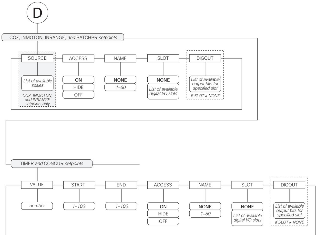
Figure 8-5. COZ, INMOTON, INRANGE, and BATCHPR Setpoint Parameters
