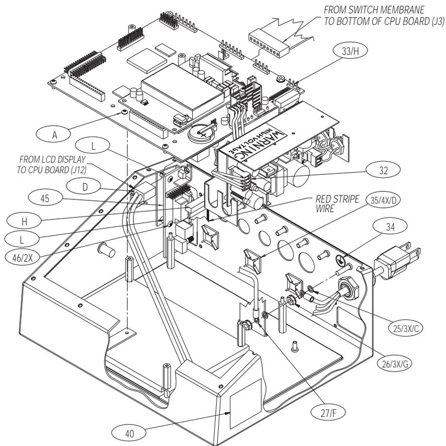
Figure 2-19. 920i Universal Model Power Supply Components
