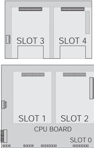
Figure 2-7. CPU Board with Two-Card Expansion Board
