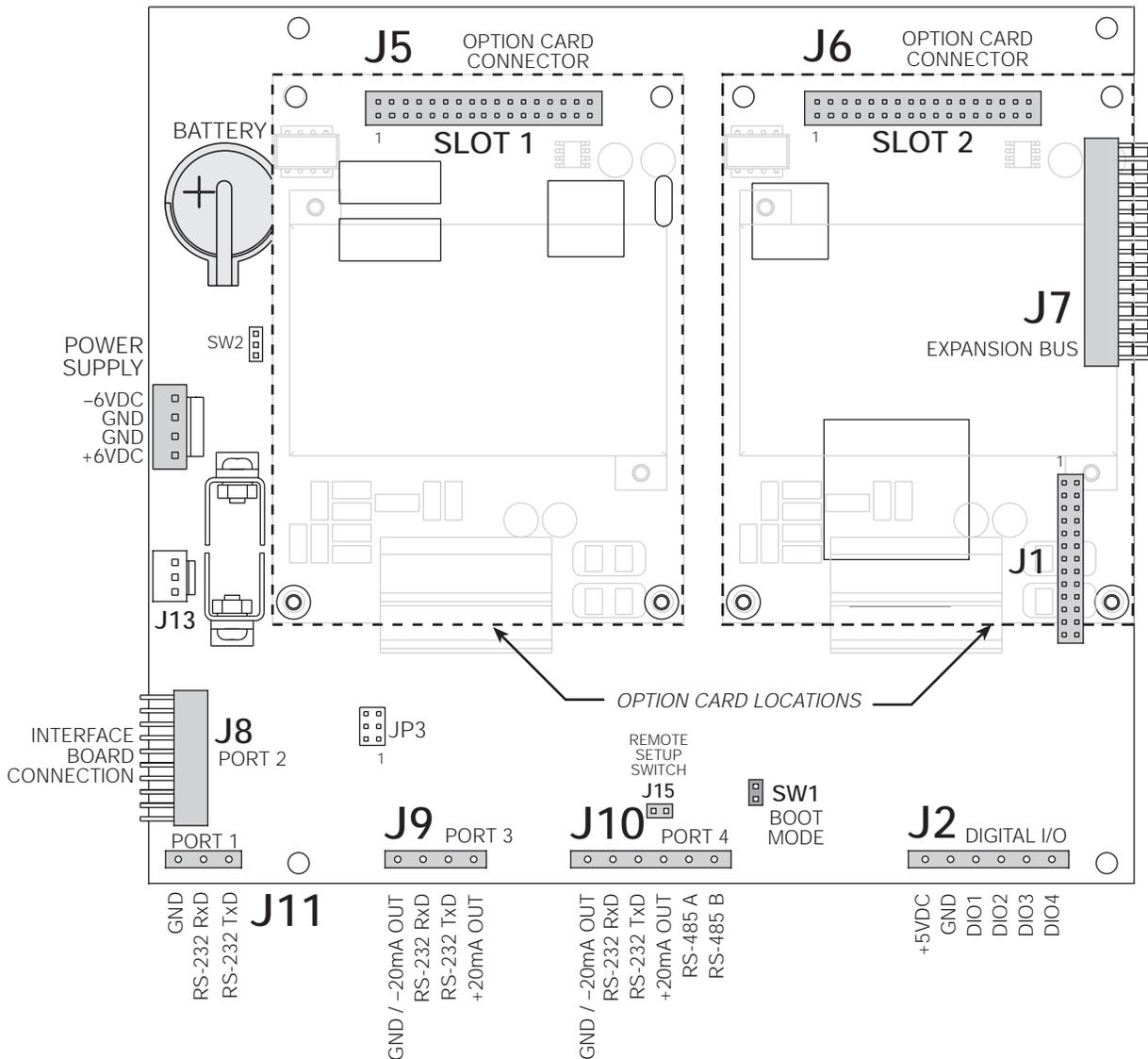
Figure 2-4. 920i CPU Board, Showing Option Card Locations
