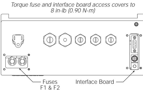
Figure 2-13. Interface Board and Fuse Locations, Universal Model
