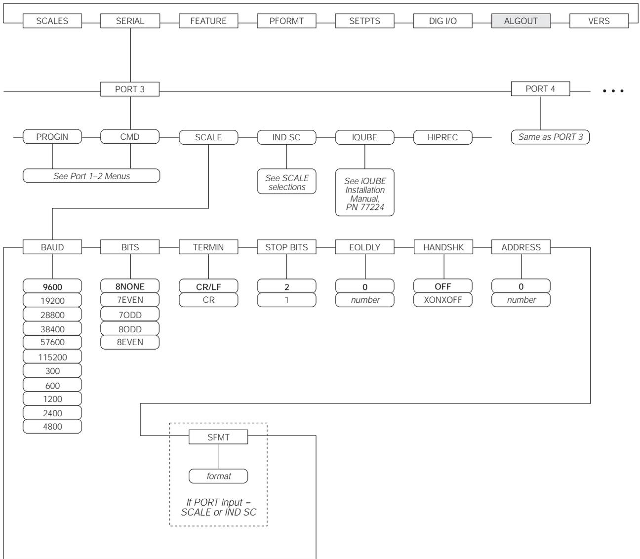
Figure 3-8. SERIAL Menu, Ports 3-4 and Expansion Ports
