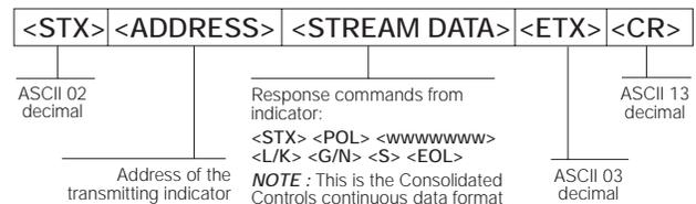
Figure 10-5. RS-485 Continuous Data Format
