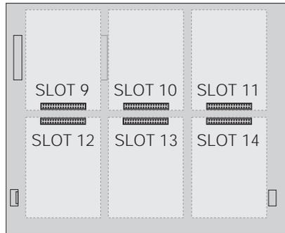
Figure 2-9. CPU Board with Two Six-Card Expansion Boards
