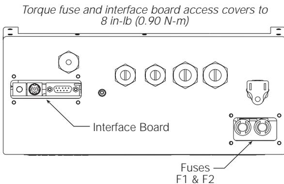
Figure 2-12. Interface Board and Fuse Locations, Desktop Model
